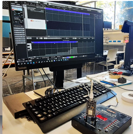
Raspberry+WiFi: knob control via wifi getting the input via WiFi, moving the knob as response. Full project here
